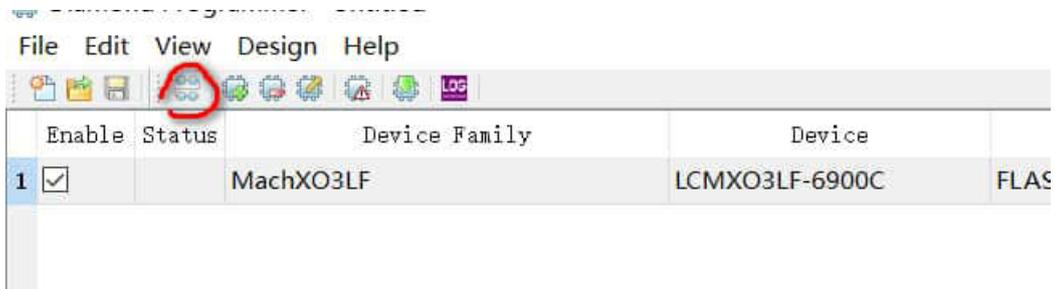
Select static ram cell mode under operation double click. Select SRAM Fast Program under operation below. , select the programming file with the suffix bit.
