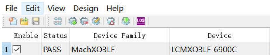
Select operation and double-click to open, i2c interface programming, select i2c program feature rows, and set the files of programming options as the corresponding modified files. Select the default address of 10000 for I2c slave address.
