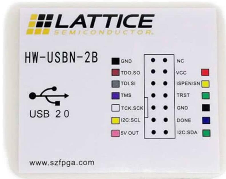
Lattice PAC-Designer software does not support Hw-USBn-2b programmers. So use HW-USBN-2B programming ispPAC chip, so Diamond Programmer or ispVM System software burned. For the newer version of Radiant, you need to install Windows10 to support the Hw-USB2-2B programmer. Side test indicator to indicate power supply, target board power supply.
