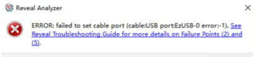
The first reason is that the simulation speed of HW-USBN-2A is too slow, which leads to the exception. Only by replacing HW-USBN-2B faster device can the root problem be solved.
